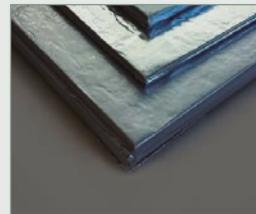
U-Vacua™ VIPs consist of a unique fiberglass core encased in a laminate film made up of several layers that include nylon, aluminium, and a protective layer. Interior pressure is reduced to a vacuum of 1-20 Pa, thereby minimizing thermal conductivity.
