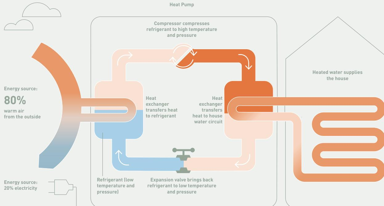
With Aquarea up to 80% of the heat energy required is taken from the ambient air. Aquarea captures heat energy from the ambient air and transfers it to heat the water needed to warm your home for domestic hot water and even to cool the house if wished.
