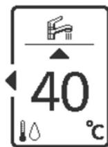
Use the UP or DOWN button to change the tank set temperature.
